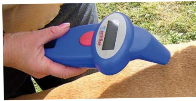
**Scanning for a microchip implant: in cold weather, some implanters have reported that some scanners do not work efficiently unless warm enough.**
